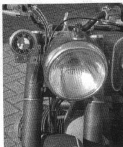
Above: Telescopic forks were another BMW innovation dating back some years; ironically, they moved away from 'teles' in favour of Earles-type forks in 1956.
